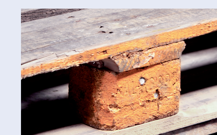
Contaminations which can be passed onto the products e.g. paint, oil, smell, mould, mould stains etc.
