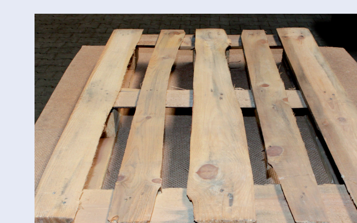
Inadmissible component e.g. under- dimensioned, woodwormeaten, wane
